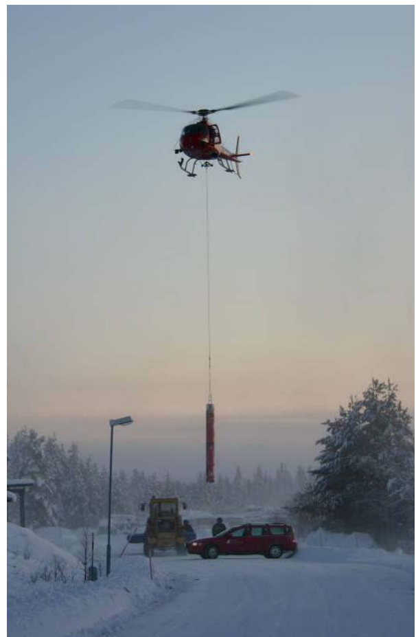
Top: MAXUS 7 payload following landing on 2 May 2006. Bottom: Helicopter retrieving a sounding rocket payload following landing (Images: SSC)
