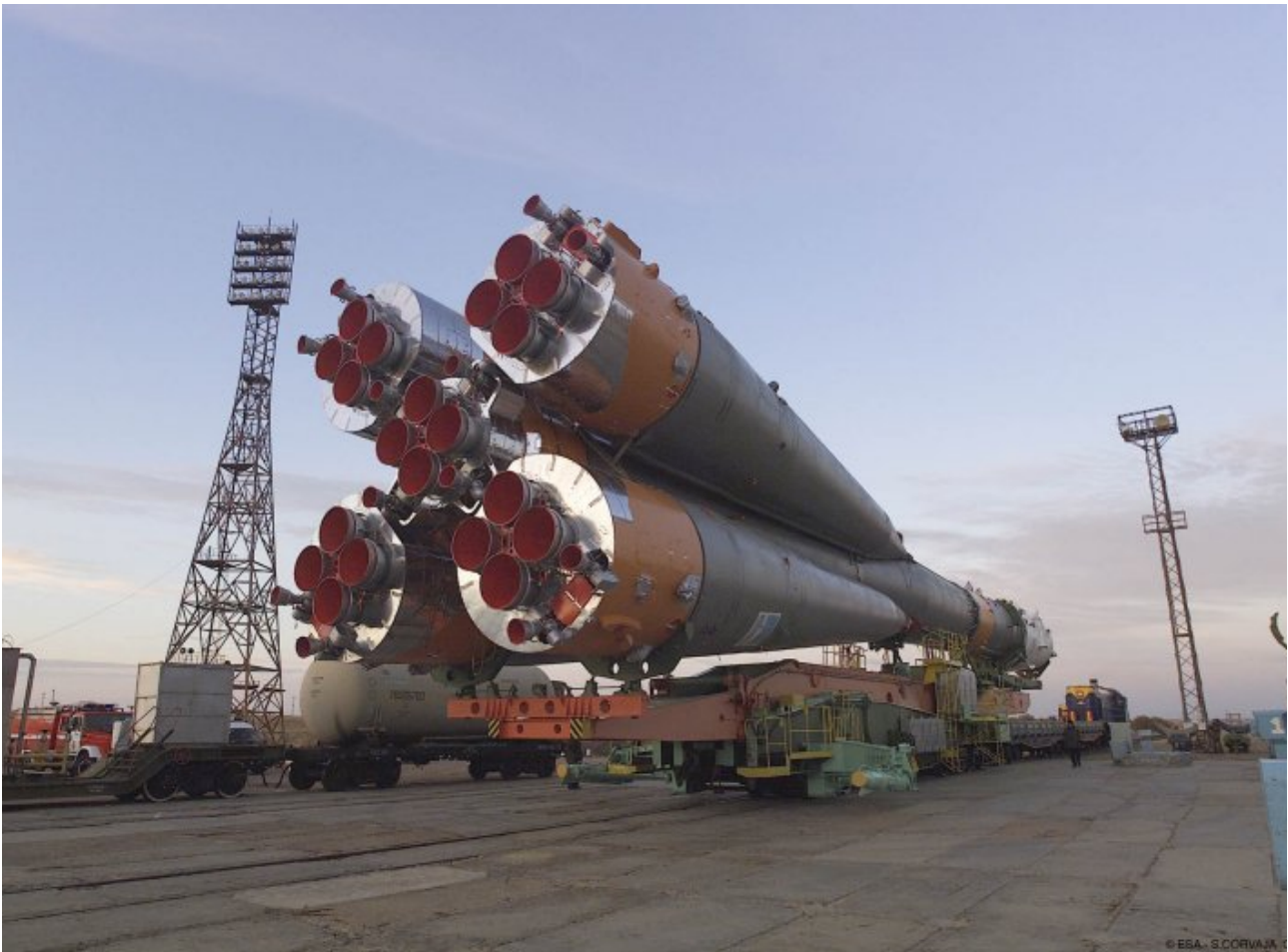
Soyuz launcher with clear view of lateral boosters arranged around central core stage (Image: ESA/S. Corvaja)
