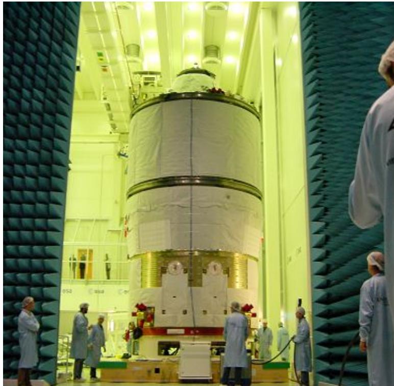
The 1 st ATV flight model (Jules Verne being moved into the Maxwell electromagnetic radiation chamber)
