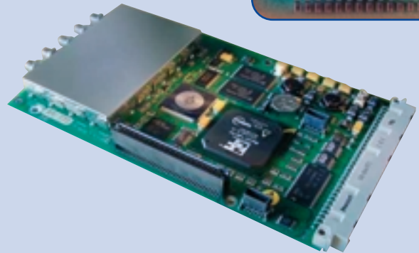
Dual frequency high performance GNSS Rx Board (Courtesy: Septentrio)
