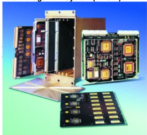
The European-built Data Management System. (Image: ESA)
