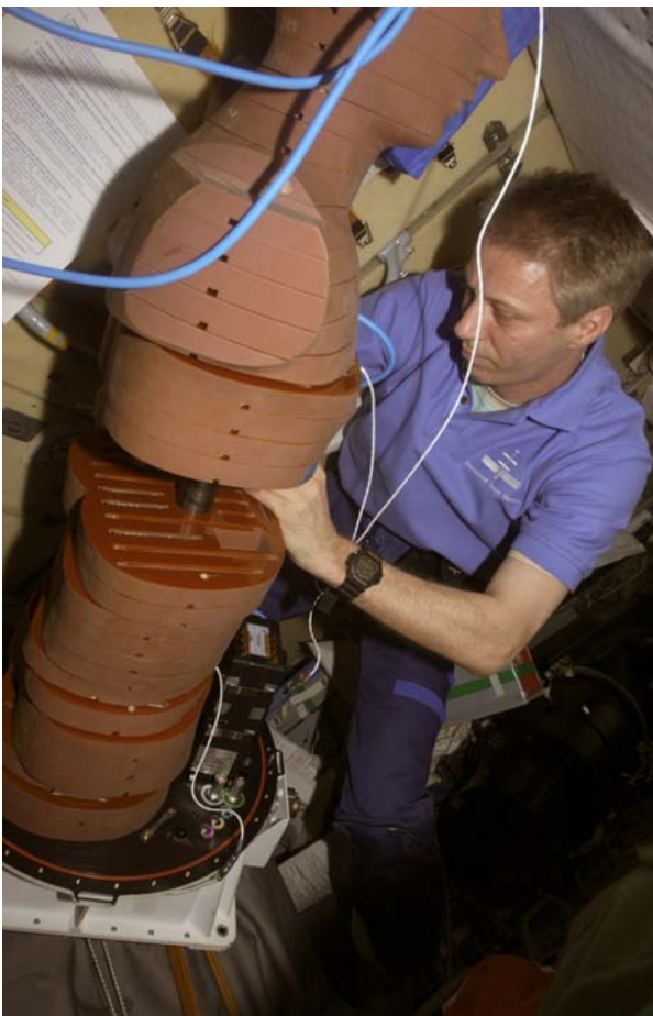
ESA astronaut Thomas Reiter inserting radiation sensors in the European Matroshka experiment in December 2006 in the Zvezda Service Module on the ISS. (Image: NASA)
