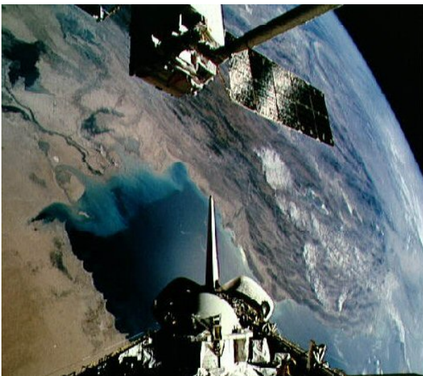
ESA's European Retrieval Carrier (EURECA) being held by the Shuttle's robotic arm prior to deployment on STS-46 Shuttle mission in 1992. (Image: NASA)
