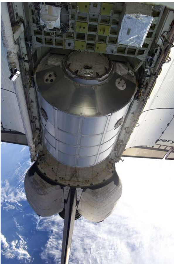
First European-built Multi-Purpose Logistics Module on orbit in Discovery's cargo bay during STS-102 mission on 10 March 2001. Node 2 follows the same structural concept as the MPLMs. (Image: NASA)
