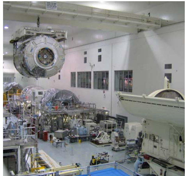
Node 2 being moved by crane in preparation for its element leak test in February 2005. (Image: NASA)
