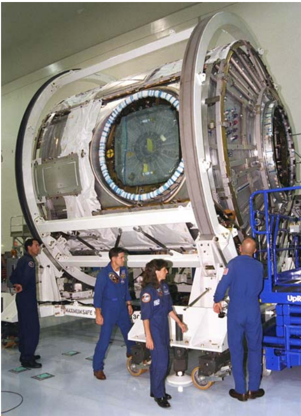
Members of the STS-88 crew examine Node 1 in the Space Station Processing Facility in June 1997. Node 2 originally had the same design though this was revised following ESA taking responsibility for its development in 1997. (Image: NASA)
