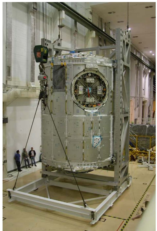
Node 2 in preparation for its element leak test in February 2005. (Image: NASA)
