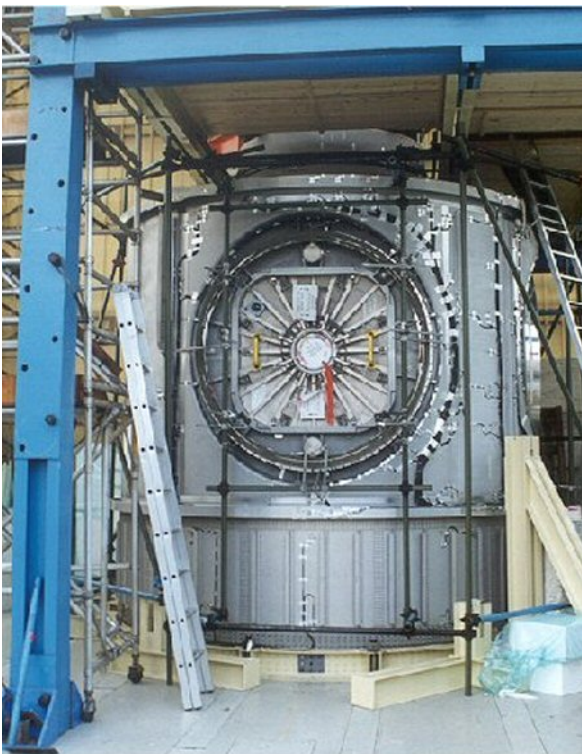
Node 2 Structural Test Article during testing. (Image: Thales Alenia Space)
