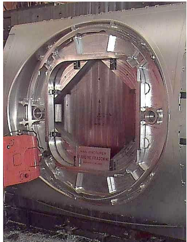
Node 2 Structural Test Article radial bulkhead during final machining in Turin in October 1998. (Image: Thales Alenia Space)
