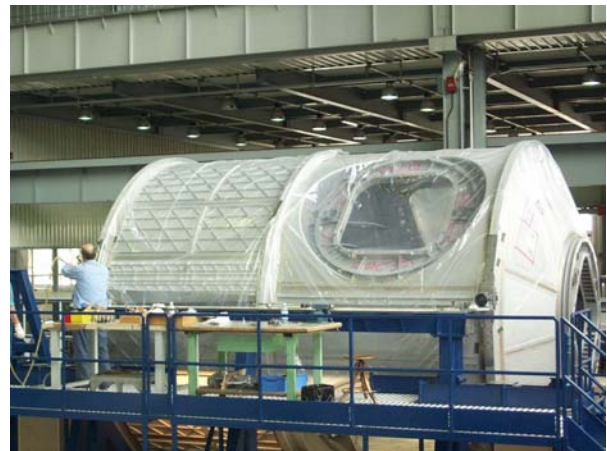
Node 2 primary structure. (Image: Thales Alenia Space)
