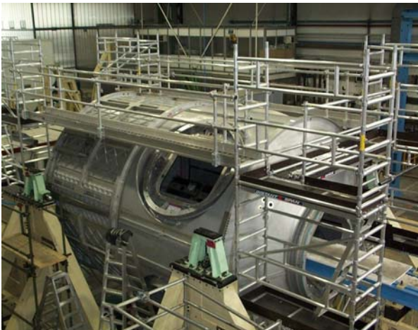
Node 2 during Modal Survey Test on 13 July 2001. (Image: Thales Alenia Space)
