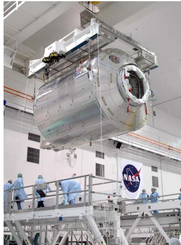
The European Columbus laboratory being lowered onto a workstand at the Space Station Processing Facility at the Kennedy Space Center in June 2006. (Image: NASA)
