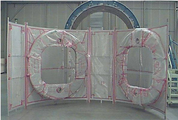
Two radial bulkheads following welding in June 1999. (Image: Thales Alenia Space)
