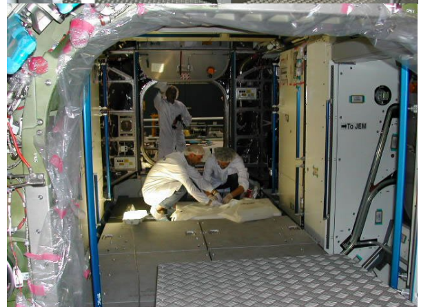
Node 2 in the Alenia integration hall in Turin, Italy for final test, integration and verification: (Top) during Micrometeoroid and Debris Protection panels installation; (Bottom) during close-out procedures prior to shipment. (Image: Thales Alenia Space)
