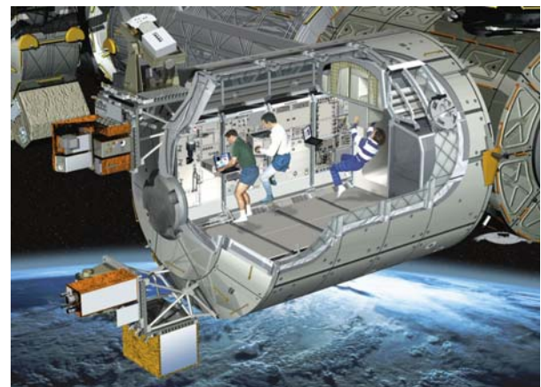
Cutaway graphic of European Columbus Laboratory attached to the ISS. The STS-122 mission in December will transport this laboratory to the ISS in the Shuttle's cargo bay. (Image: ESA/D. Ducros)
