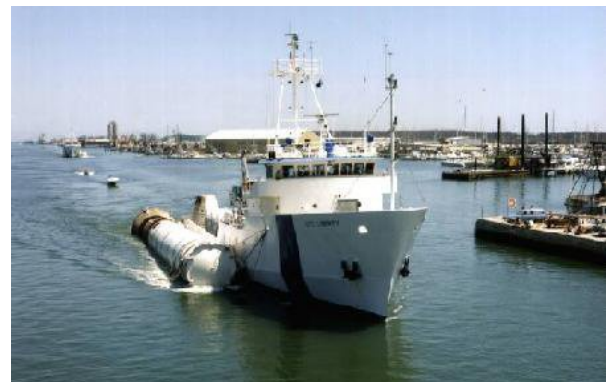
Recovery vessel towing Solid Rocket Booster casing. (Image: NASA)
