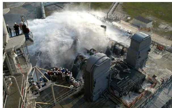
Sound Suppression System test on launch pad 39A at the Kennedy Space Center. (Image: NASA)
