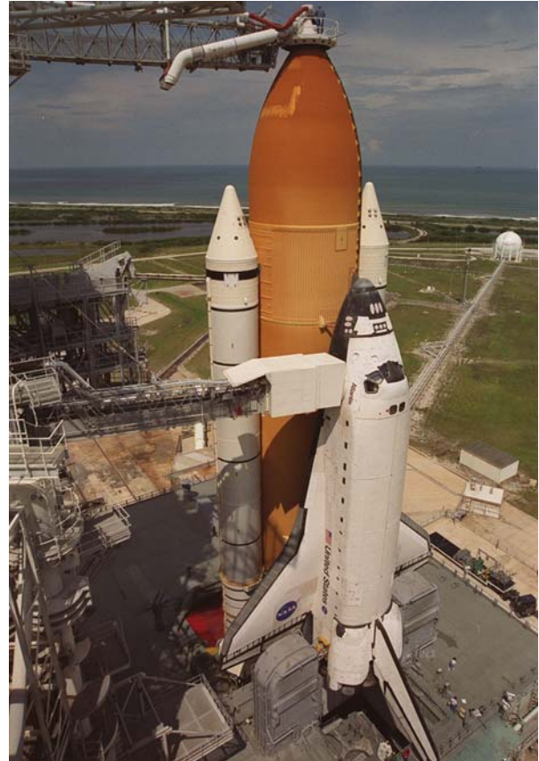
STS-106 on launch pad. White Room is attached to the orbiter at the end of the Orbiter Access Arm. The beanie cap is shown at the top of the External Tank prior to removal. (Image: NASA)
