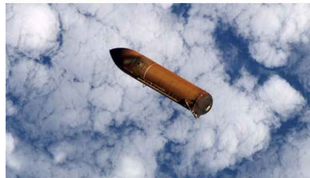
External Tank from the STS-114 Return to Flight mission following jettison. (Image: NASA)
