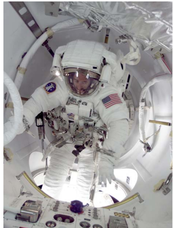
NASA astronaut James Reilly leaves through the Joint Airlock Quest during the first ever spacewalk from the International Space Station in July 2001. Clear view of Umbilical Interface Assembly at bottom of photo. (Image: NASA)
