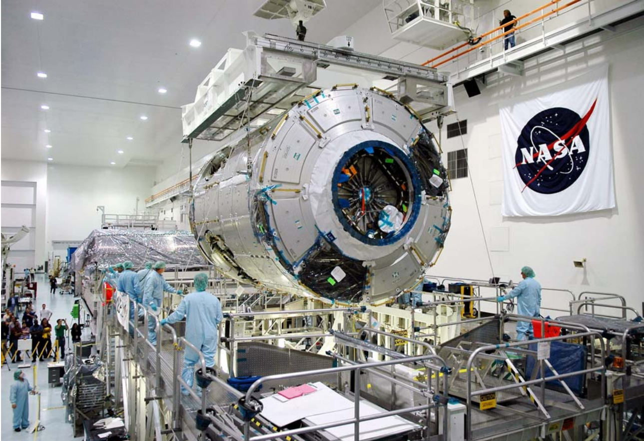
The European-built Node 2 being lifted from its work stand in the Space Station Processing Facility at the Kennedy Space Center in the United States. The module was being transferred in order to undergo an element leak test. This image shows a clear view of the aft docking mechanism where Node 2 will ultimately be attached to the ISS at the US Destiny laboratory. (Image: NASA)
