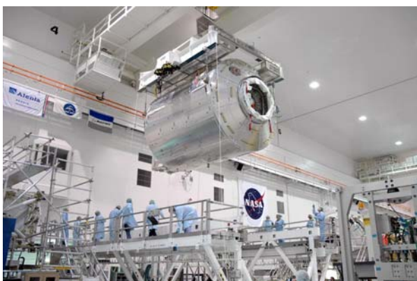
European Columbus laboratory being lowered onto a work stand at the Kennedy Space Center. Columbus is due for launch and attachment to Node 2 in December 2007. (Image: NASA)
