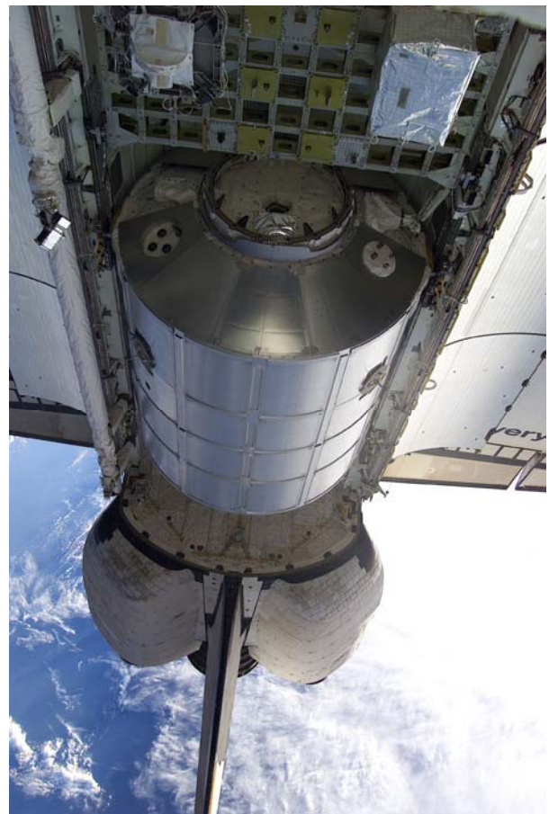
Multi-Purpose Logistics Module Leonardo in the Space Shuttle cargo bay on 10 March 2001 during the STS-102 mission to the ISS. Node 2 shares its basic structure with the Multi-Purpose Logistics Modules and will travel to the ISS in a similar fashion. (Image: NASA)
