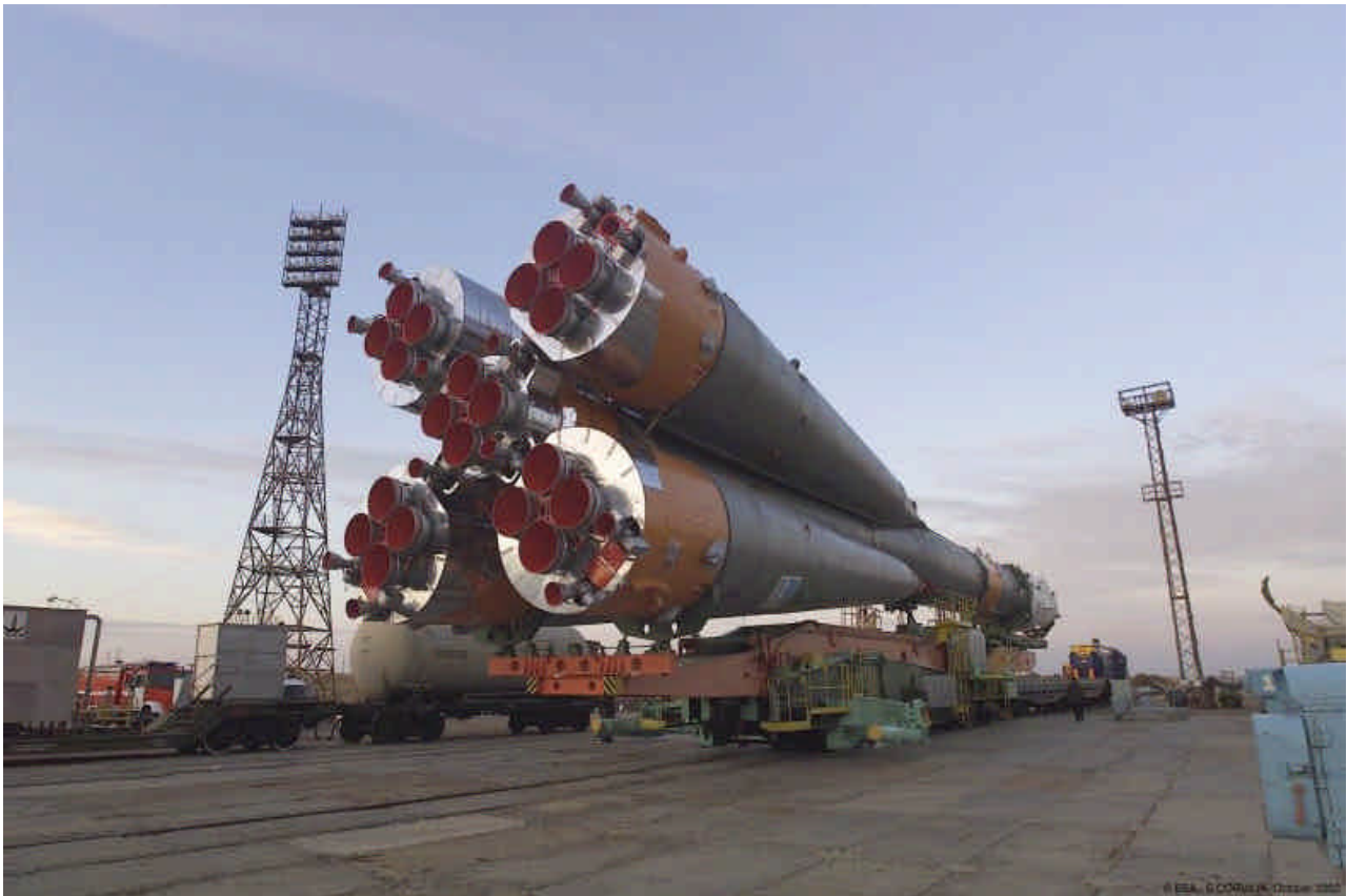
Soyuz launcher with clear view of lateral boosters arranged around central core stage
