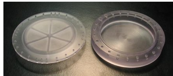
Bone proteomics experiment culture chamber (Image: ESA)
