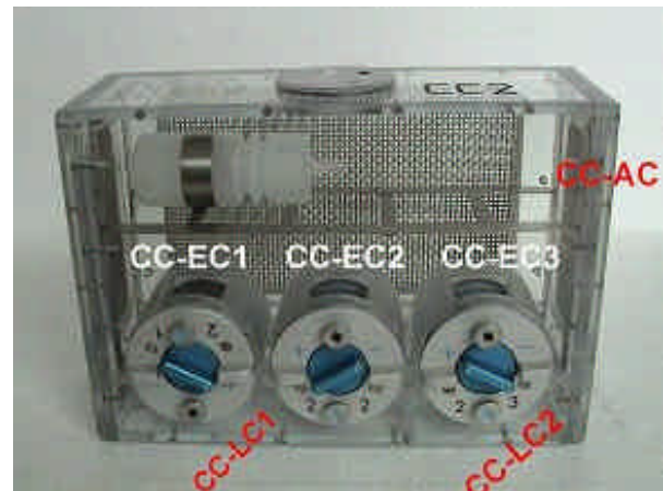
One of the two Experiment containers, showing the adult compartment (CC-AC), the egg collectors (CC-EC) and hatching larvae compartments (CC-LC) (Image: E. Horn)
