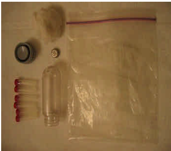
Hardware set: Sigma centrifuge tubes, cryo-vials, smart button, microbiological cotton, Ziploc bag (Image: F. Cangarella)
