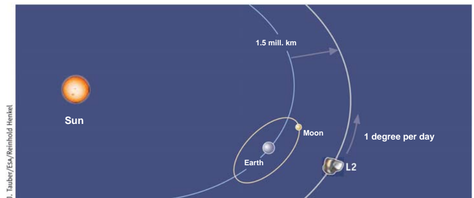
▶ Fig. 5: Planck rotates once a minute around an axis that is pointed away from the Sun. The field of vision is inclined 85 degrees from the rotational axis and therefore covers a circular band in the sky when rotating. While Planck is following its path around the L 2 and around the Sun this circular band covers the entire sky within six to seven months (far right).
