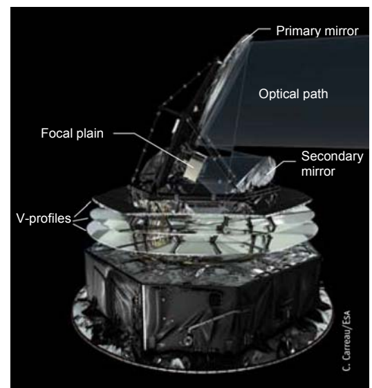
Fig. 11: The Planck telescope collects the radiation from the sky and bundles it in the focal plane. It is a total of three metres high and three metres wide, and its two aluminised mirrors consist of carbon fibre reinforced plastic.
