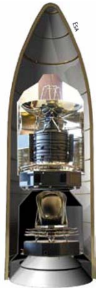
Fig. 1: Herschel and Planck are housed in an Ariane 5 rocket ready for launch. Soon after the launch they will continue separately on their journey.
