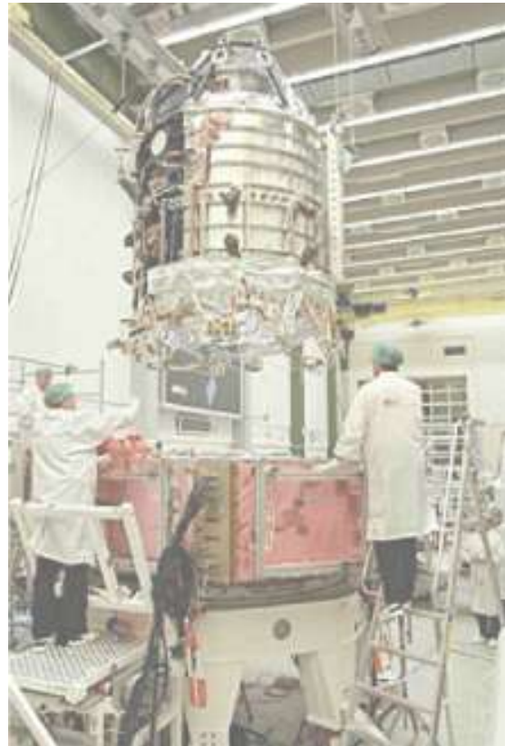
Fig. 7: Cryostat and service module of the Herschel space telescope. (Picture: http://www.esa.int/esaSC/SEM0ZJPK6F_index_0.html )
