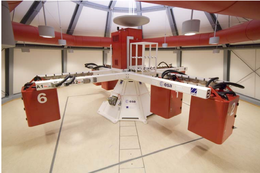
Large Diameter Centrifuge
