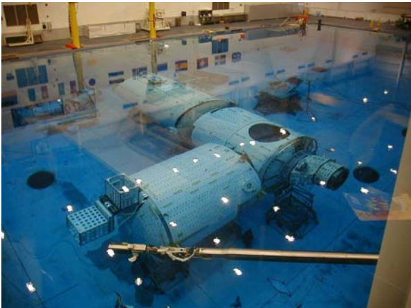
Columbus Neutral Buoyancy testing at Johnson Space Center, USA.
