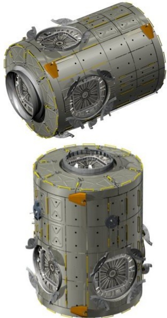
ESA-developed Node 2 (top), the attachment point of the Columbus Laboratory and Node 3 (bottom). Node 3 will be the attachment point of the Cupola. (Image: ESA/D.Ducros)
