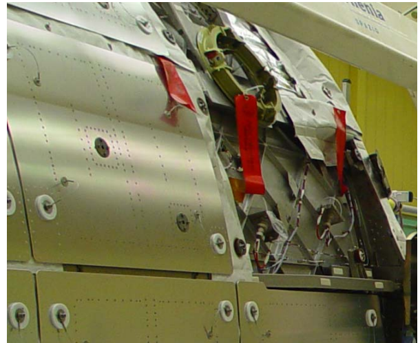
Close up of Columbus with Meteoroid and Debris Protection System panels. One panel removed along with thermal blanket layer to reveal primary structure. (Image: EADS Astrium)
