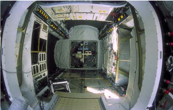
Fisheye photo of Columbus with flight models of the European experiment facilities installed during testing in 2004.
