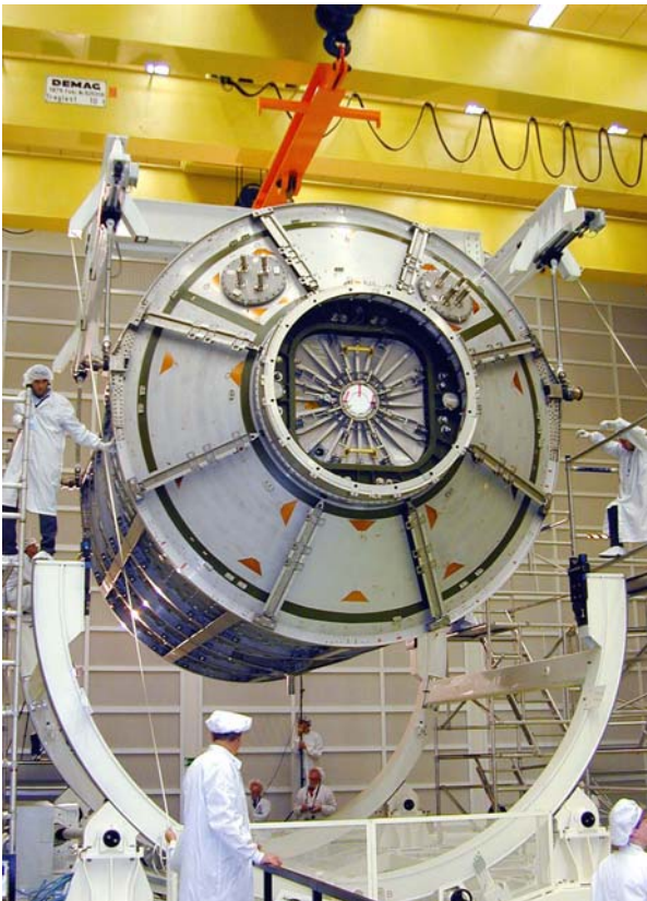
The Pre-integrated Columbus Assembly (PICA) being lowered onto the Columbus integration stand at EADS in Bremen after arrival from Alenia Spazio in Turin. (Image: EADS Astrium)
