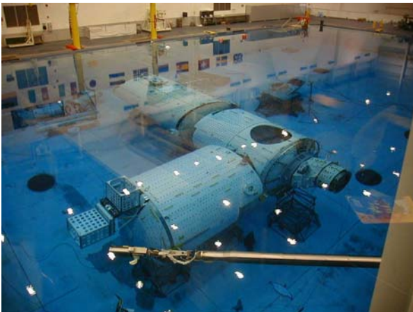
Columbus Neutral Buoyancy testing at the Johnson Space Center in the USA in 2000.
