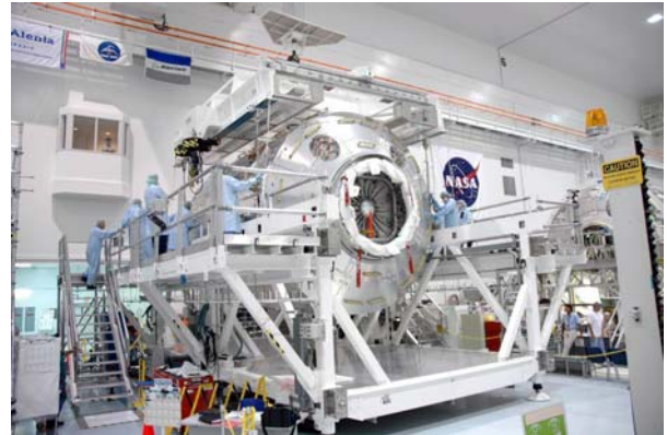
Columbus laboratory on a workstand in the Space Station Processing Facility of the Kennedy Space (Image: NASA)
