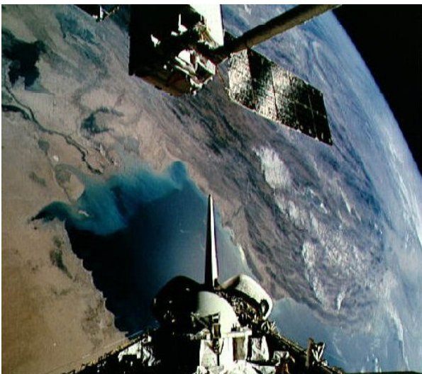
ESA's European Retrievable Carrier (EURECA) being held by the Shuttle's robotic arm prior to deployment on STS-46 Shuttle mission in 1992. (Image: NASA)
