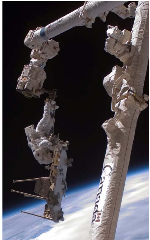
ESA astronaut Christer Fuglesang during the second EVA on the ISS 12A.1 assembly mission in December 2006. Attached by a footplate to the Station's robotic arm, Fuglesang is relocating a piece of EVA hardware to a different location on the ISS truss to clear the way for activities on the third EVA. (Image: NASA)
