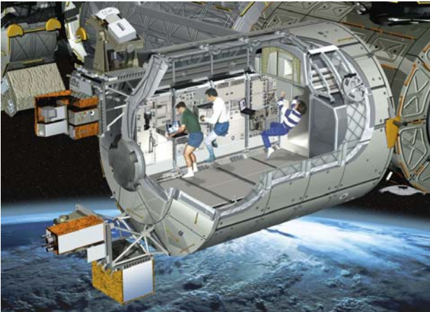
Cutaway graphic of European Columbus Laboratory attached to the ISS. The STS-122 mission in February 2008 will transport this laboratory to the ISS in the Shuttle's cargo bay. (Image: ESA/D. Ducros)
