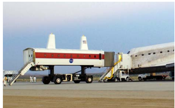
Crew Transport Vehicle pulls up to Space Shuttle Discovery to offload the crew following landing of the STS-114 mission. 9 August, 2005. (Image: NASA)
