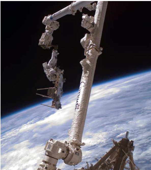
ESA astronaut Christer Fuglesang being moved by robotic arm during an EVA as part of the STS-116 (12A.1) ISS assembly mission. (Image: NASA)
