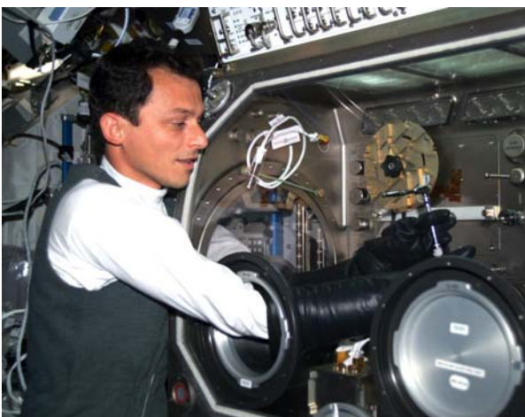
Former ESA astronaut Pedro Duque works on the PROMISS experiment inside the Microgravity Science Glovebox during the Cervantes mission in October 2003. (Image: ESA/P. Duque)
