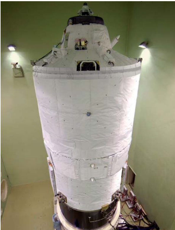
ATV during acoustic test campaign (Image: ESA/S.Corvaja)
