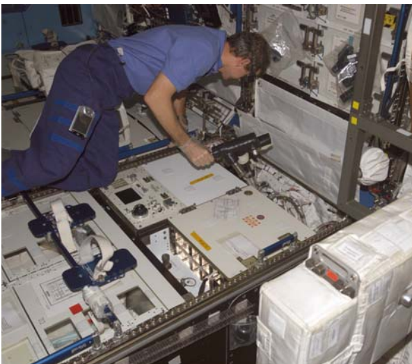
Maintenance Operations: Expedition 12 Commander Bill McArthur preparing to remove the Avionics Air Assembly from the Crew Health Care System (CHeCS) rack on 9 December 2005. (Image: NASA)
