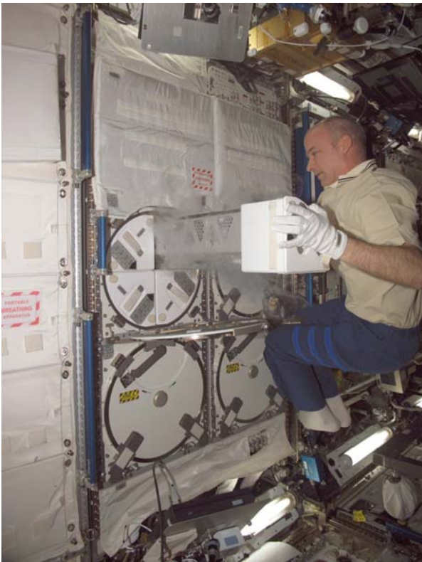
NASA astronaut and Expedition 13 Flight Engineer Jeffrey Williams inserts a sample into the Minus Eighty Degree Laboratory Freezer for ISS (MELFI) on the International Space Station on 2 Aug. 2006. (Image: NASA)
