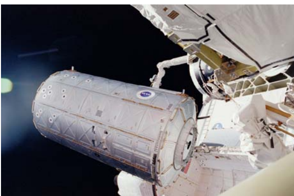
The US Destiny laboratory being moved by robotic arm from Shuttle Atlantis' cargo bay during the STS-98 mission in February 2001 (Image: NASA)
