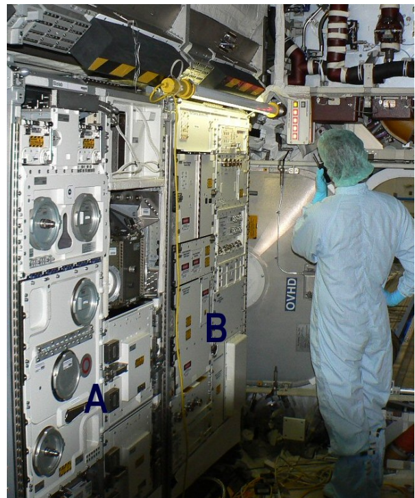
Biolab (A) and the Fluid Science Laboratory (B) integrated into the European Columbus laboratory at the Kennedy Space Center.
