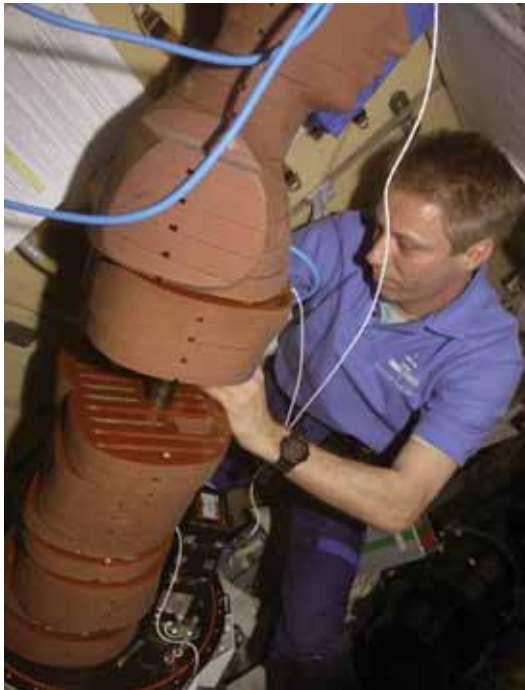
ESA astronaut Thomas Reiter, working with the European Matroshka on the ISS. Matroshka, which simulates a human torso, has been used since February 2004 to measure radiation dosage outside and, at the moment, inside the ISS.
