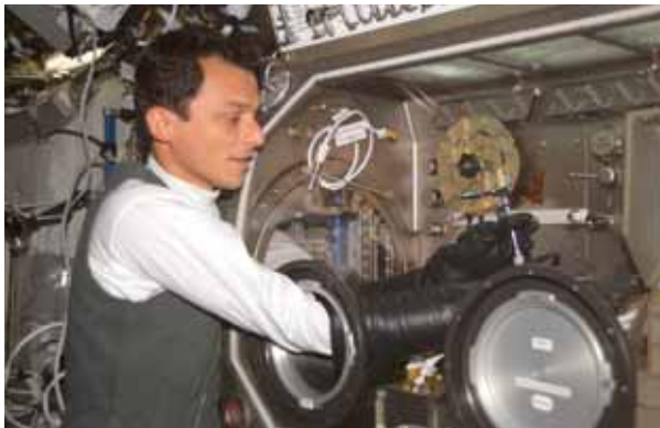
ESA astronaut Pedro Duque working on the PROMISS experiment in the European-built Microgravity Science Glovebox on the ISS. PROMISS used advanced optical diagnostics to investigate the growth processes of proteins during weightless conditions.
