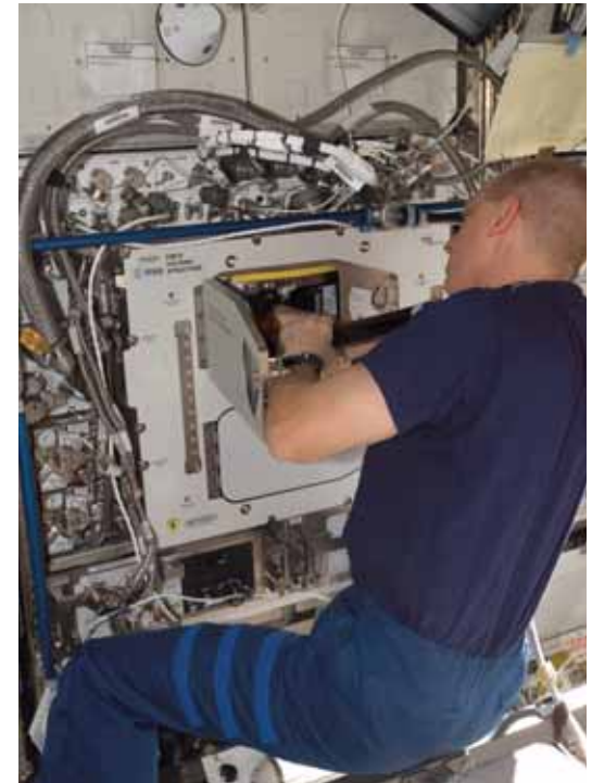
NASA astronaut Clay Anderson working with the European Modular Cultivation System (EMCS) on the ISS in July 2007. The facility is undertaking biological experiments, principally addressing the effects of gravity on plant cells, roots and physiology.
