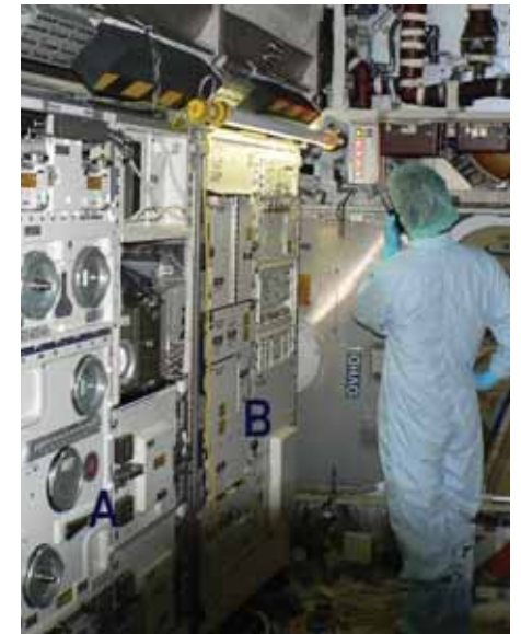
Two of the major ESA research facilities installed in Columbus: (A) Biolab, for biological experiments, and (B) the Fluid Science Laboratory (FSL).
