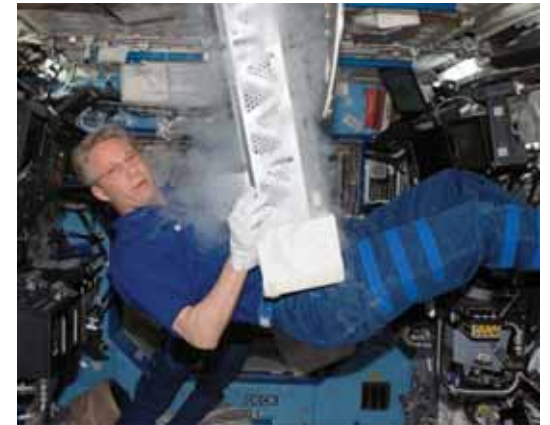
ESA astronaut Thomas Reiter handling an insert from the European-built Minus Eighty Degree Laboratory Freezer for the ISS (MELFI), used to store sensitive life science samples at low temperatures.
