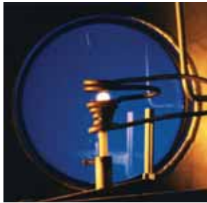
The Electromagnetic Levitator, jointly developed by ESA and the German space agency, permits the accurate measurement of the properties of highly reactive liquid metal alloys. It will be flown to the ISS after 2008.
