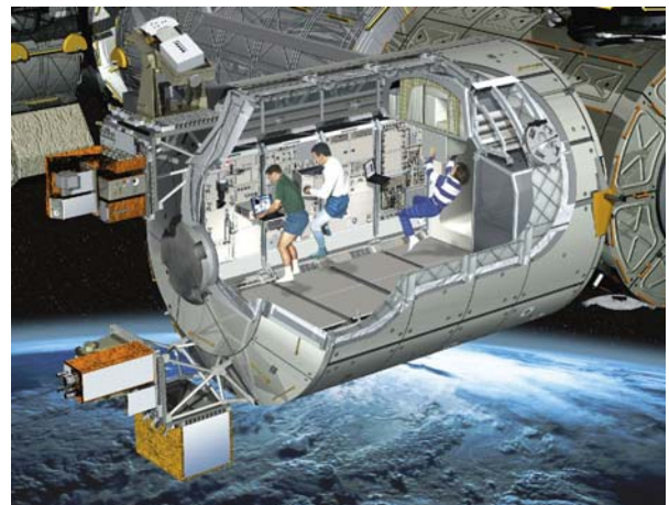
Cutaway graphic of European Columbus Laboratory attached to the ISS. A subsequent Shuttle mission will transport this laboratory in the Shuttle's cargo bay. (Image: ESA/D. Ducros)
