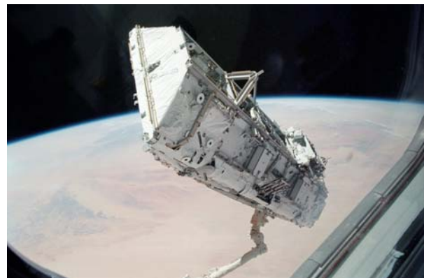
The S0 truss being moved outside of Space Shuttle Atlantis' cargo bay by the ISS robotic arm during the STS-110 mission on 11 April 2002. (Image: NASA)
