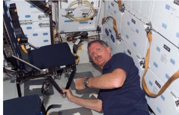
NASA astronaut Joseph Tanner prepares to remove a launch and entry seat on mid deck of Atlantis soon after the Crew reached Earth orbit on flight day 1 of the STS-115. (Image: NASA)
