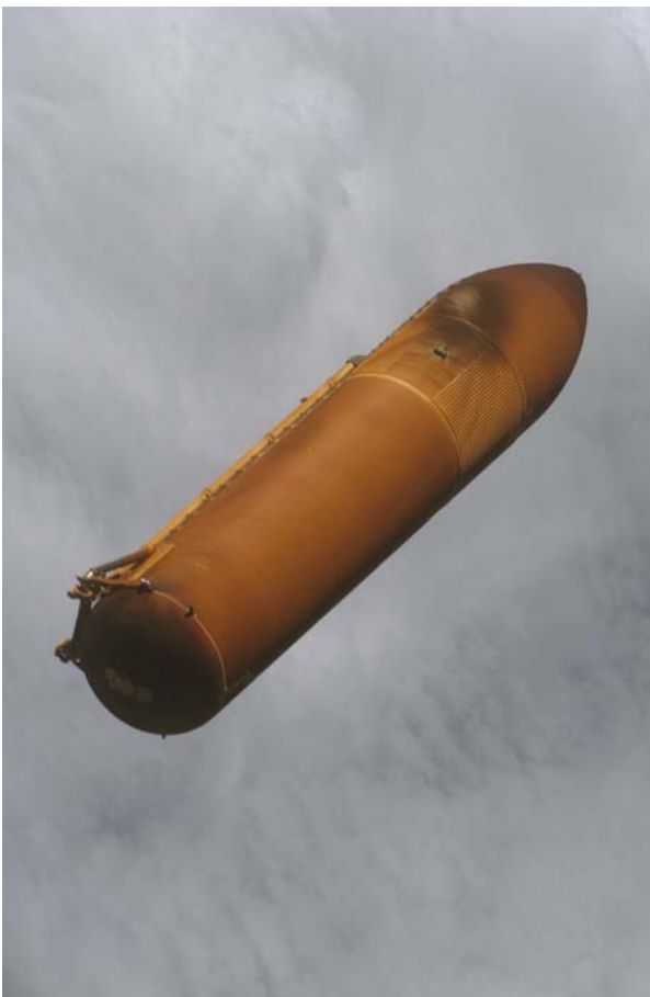
STS-115 external tank after separation from the Space Shuttle Atlantis on 9 September 2006. A crew member onboard the shuttle recorded the image with a digital still camera. (Image: NASA)
