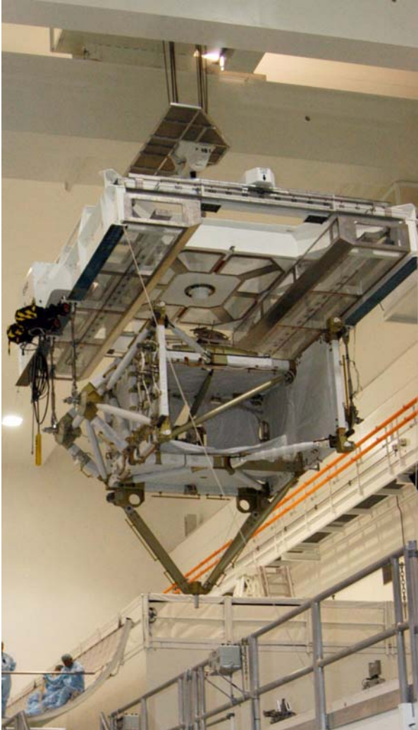
The P5 truss section being moved by crane towards the payload canister (out of shot) in the Space Station Processing Facility of the Kennedy Space Center in Florida in October 2006. The canister will be used to transport the truss to the launch pad for loading into the Shuttle cargo bay. (Image: NASA George Shelton)
