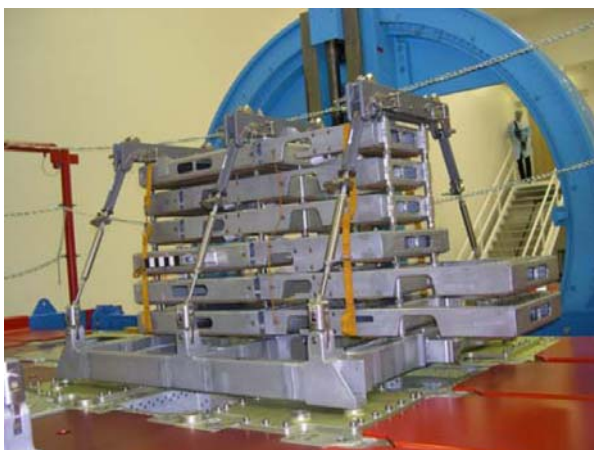
Bundle of Service Module Debris Panels in fixation device.
