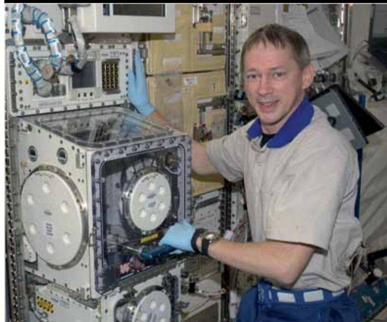
Frank De Winne works with the Space Linear Acceleration Mass Measurement Device (SLAMMD) in Europe's Columbus laboratory. SLAMMD is used to determine the body mass of crew members as part of ongoing medical investigations.
