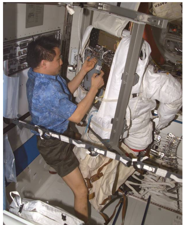
NASA astronaut Ed Lu undertaking periodic maintenance of an EMU in the Quest Airlock. (Image: NASA)
