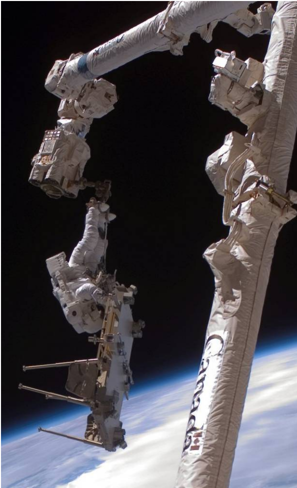
ESA astronaut Christer Fuglesang during the second EVA on the ISS 12A.1 assembly mission in December 2006. Attached by a footplate to the Station's robotic arm, Fuglesang is relocating a piece of EVA hardware to a different location on the ISS truss to clear the way for activities on the third EVA. (Image: NASA)
