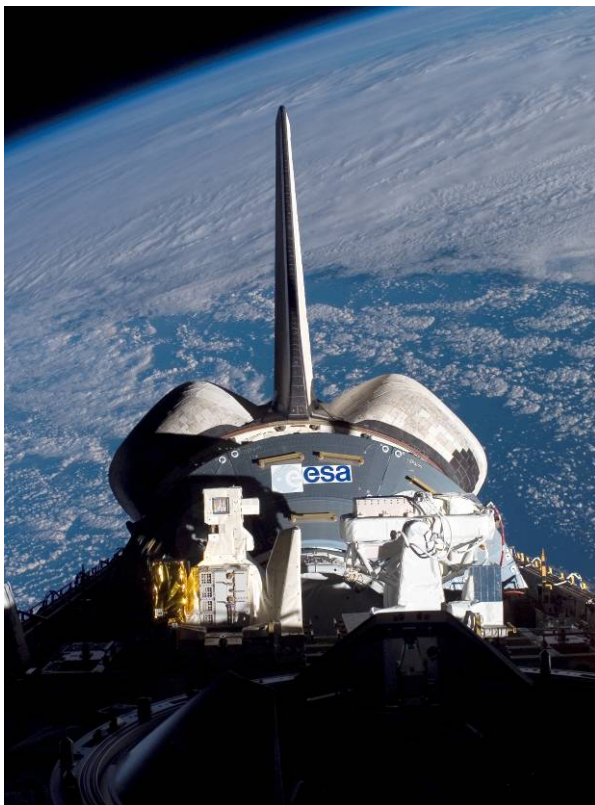
ESA's Columbus laboratory being transported to the ISS in the cargo bay of Space Shuttle Atlantis on 8 February 2008. In front of Columbus are its first two external experiment payloads SOLAR (left) and EuTEF (right) (Image: NASA)
