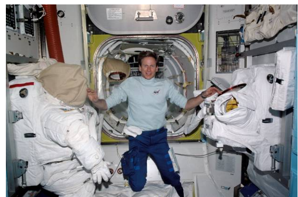
NASA astronaut Michael Gernhardt in the Equipment Lock of the Quest Airlock with EMU space suits during the STS-104 mission to the ISS (12-24 July 2001). On the right is the upper torso section, which contains the life support systems. (Image: NASA)
