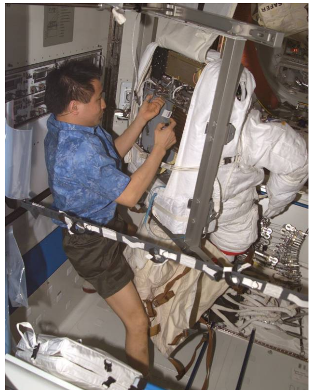
NASA astronaut Ed Lu undertaking periodic maintenance of an EMU in the Quest Airlock. (Image: NASA)
