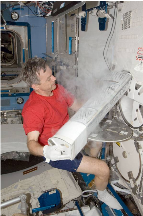
Canadian Space Agency astronaut and Expedition 20 Flight Engineer Robert Thirsk inserting samples into the European-built Minus Eighty degree Laboratory Freezer for the ISS MELFI in the Japanese Kibo laboratory. (Image: NASA)
