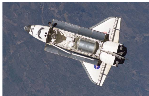
STS-121 Space Shuttle Discovery prior to docking with the ISS on 6 July 2006. The mission transported an MPLM (clear to see in Shuttle cargo bay) as well as ESA astronaut Thomas Reiter to become the first European ISS Expedition crew member (Image: NASA)
