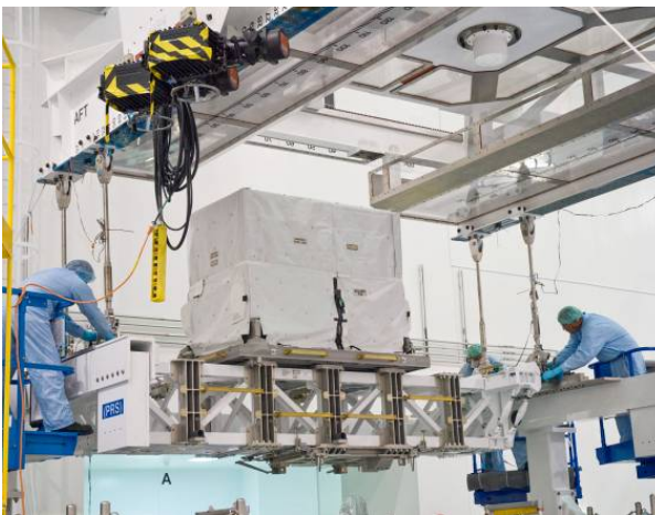
Ammonia Tank Assembly attached to the support structure that will be transported in Discovery's cargo bay for the STS-128 flight. Photo taken as workers attach a crane to the support structure at the Kennedy Space Center on 9 July 2009 (Image: NASA)
