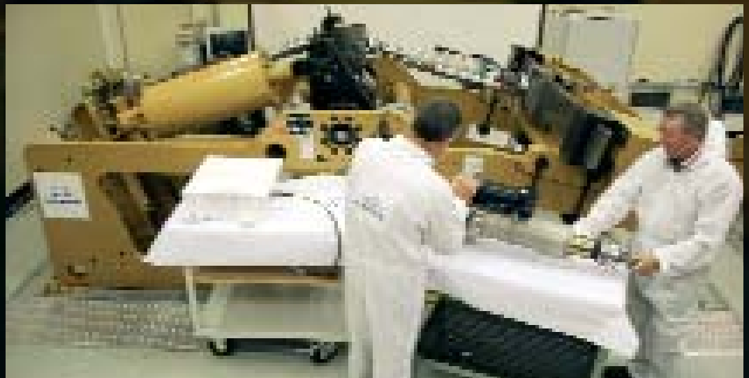
P80 TVC on the test stand
