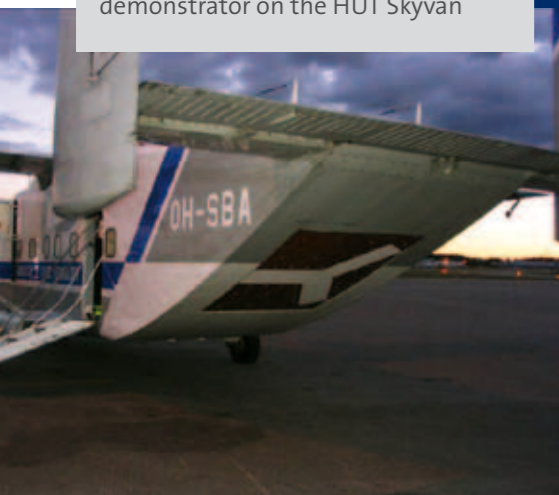
AMIRAS: the Airborne MIRAS demonstrator on the HUT Skyvan
