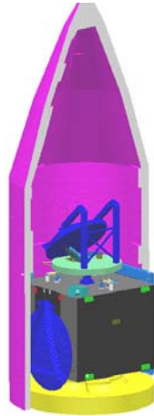
Figure 4.10: Example of GPM accommodation inside Rocket
