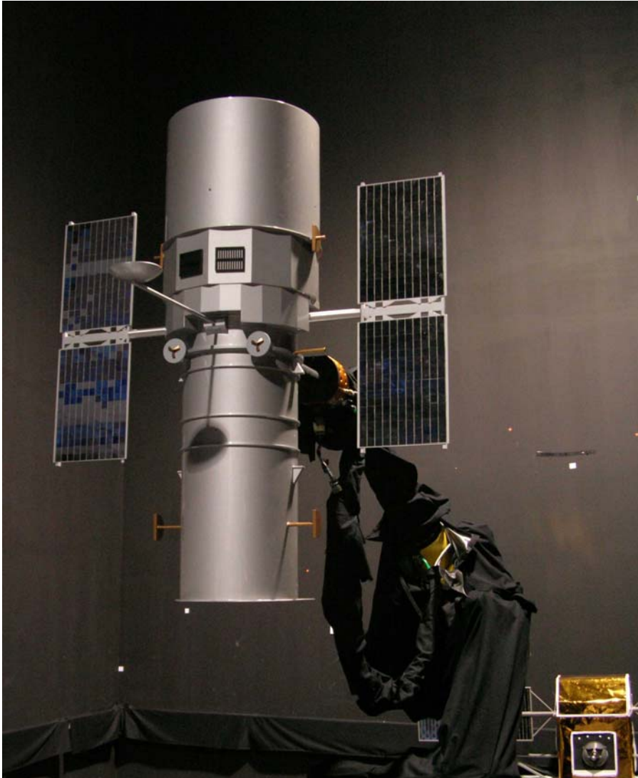
Figure 11: Scaled Rendezvous Testing of HST
